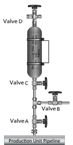
Select sampling cylinders with appropriate volume according to the required sample quantity.
